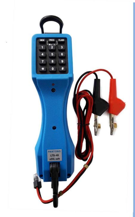
•Heavy duty butt set with High impact Nylon 6/6 case and Built-in high volt protection circuit. All operation modes( TALK/ MONITOR/ RING ) are Data safe not disrupt data service Mode selection DTMF / Pulse Line Polarity independent with Pole Indicator High Shock/Drop Resistance Last Number Redialing 10 Memories for speed dial Mute •Flash Data Safe High Impedance Monitoring. Off-hook xDSL Datasafe •Non-conductive safety design by high impact plastic Belt Clip and Hanging Loop
